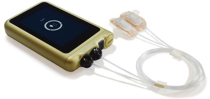
The iLet is — as envisioned — a portable, wearable electronic device, which is not much larger than the original 2007 iPhone, that takes blood-sugar readings every five minutes, and, depending on levels, either releases insulin to bring blood sugar down or glucagon to bring it back up. Damiano's goal is to have an insulin-only version of the iLet on the market by the time David enters his sophomore year of college in 2018.
